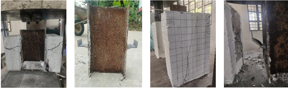
Figure 5. Failure mode of the specimen (Inverted & Normal Channel Connector Angle Connector).
