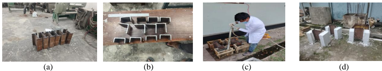
Figure 2. (a) I-steel beam, (b) Channel & angle connectors, (c) Specimen casting and (d) Specimen
