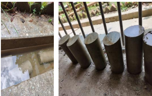
Figure 6. Curing of Specimen
