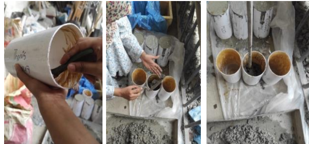
Figure 5. Mold Preparation and Casting
