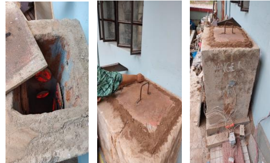
Figure 7. Thermal Exposure of Specimen
