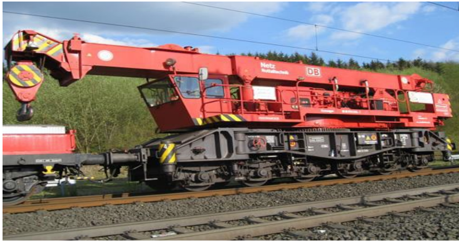
Figure 5. Multi-purpose railway crane commonly employed for switch renewal
