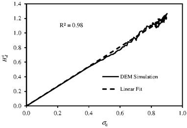
Figure 3. The relationship between the micro-quantity (fabric ratio) and macro-quantity (normalized deviatoric stress ratio) during the simulation
