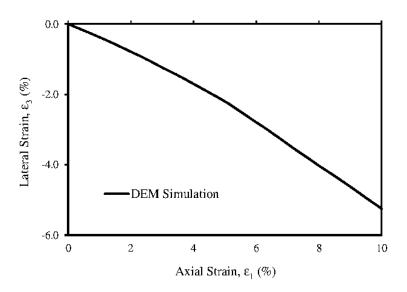
Figure 2. Relationship between the axial strain,  $\varepsilon_1$  and lateral strain,  $\varepsilon_3$  during the simulation
