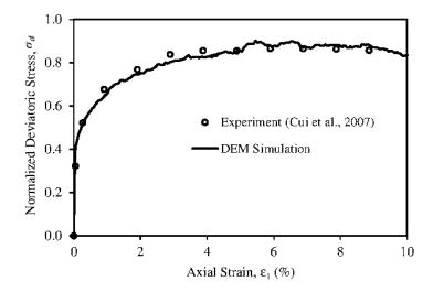
Figure 1. Comparison of the simulated stress-strain behavior with the CTC test (experiment) reported in Cui et al. (2007)
