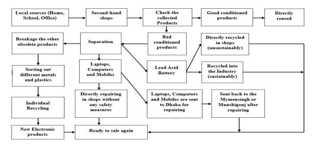
Figure 2. Qualitative flow diagram of reusing and recycling of e-waste in Mymensingh and Munshigonj
