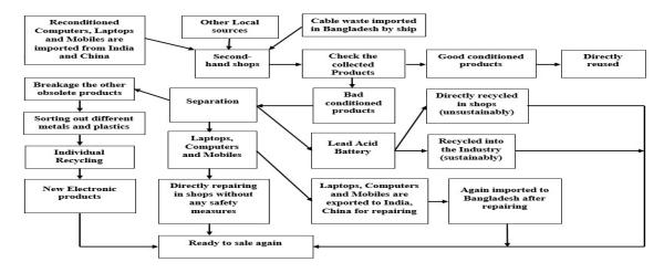
Figure 1. Qualitative flow diagram of reusing and recycling of e-waste in Dhaka City
