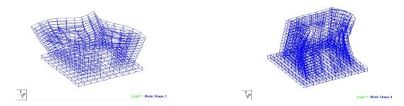
1st Torsion mode shape in Model 1 (Mode 3, 6.293 Hz) 1st Torsion mode shape in Model 2 (Mode 4, 9.166 Hz)
