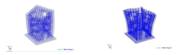
1st Torsion mode shape in Model 3 (Mode 3, 4.021 Hz) 1st Torsion mode shape in Model 4 (Mode 4, 7.11 Hz)
