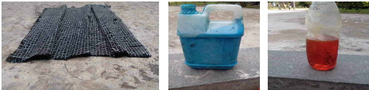
Figure 1. CFRP sheet and epoxy adhesive (primer & saturant)
