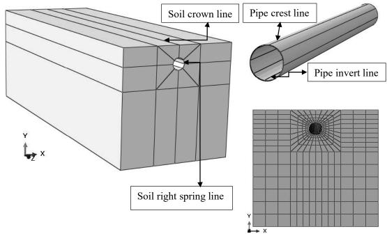
Figure 1: 3D FEM Model of Soil and Pipeline with meshing pattern (XY plane) in CAE Environment
