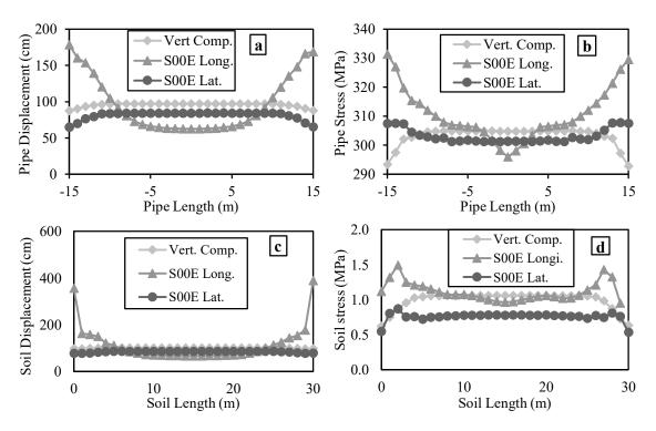
Figure 6. Seismic Response of pipe and soil (a) Max. Displacement along the pipe crest line (b) Max. Stress along the pipe invert line (c) Max. Displacement along the soil crown line (d) Max. Stress along the soil right spring line
