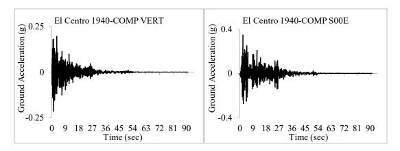
Figure 2. The accelerogram (Vertical acceleration, Transversal acceleration and Longitudinal acceleration) of the El Centro Earthquake of 18th May, 1940 (https://strongmotioncenter.org)
